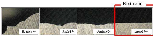
Fig. 3 Comparison of edge trimming angles.
