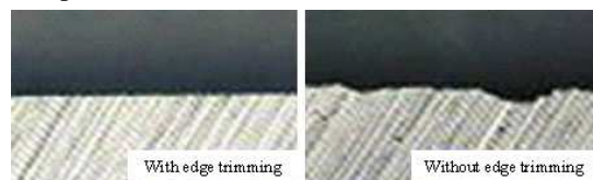
Fig. 2 Wafer edges after grinding with and without edge trimming
