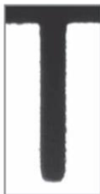
Current Kerf: 40 \mu\text{m}
